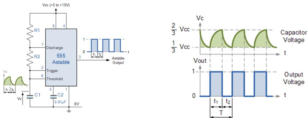
In the 555 Oscillator circuit above, pin 2 and pin 6 are connected together allowing the circuit to re-trigger itself on each and every cycle allowing it to operate as a free running oscillator. During each cycle capacitor, C charges up through both timing resistors, R1 and R2 but discharges itself only through resistor, R2 as the other side of R2 is connected to the discharge terminal, pin 7.
